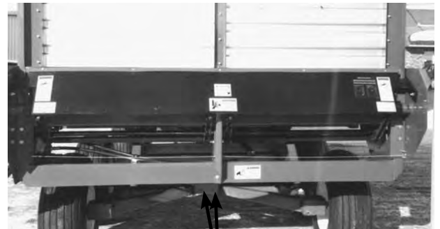
Center 2 Tightener Bolts
